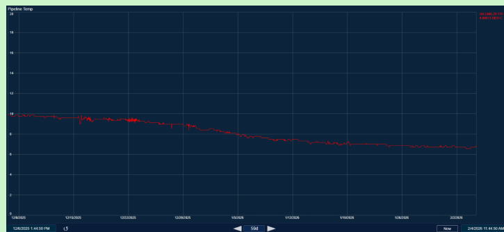
Figure 2. SEAL heater inlet temperature trends between December 2025 and February 2026. Source: PI Vision data provided by Shell UK.
